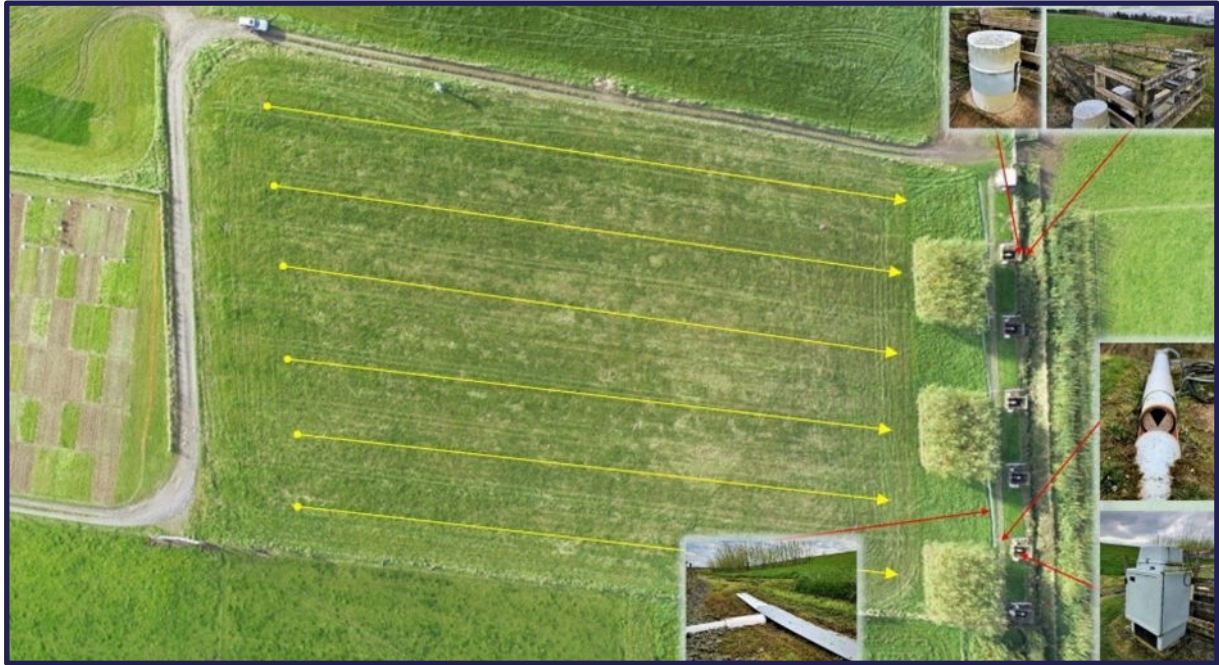
Figure 1: Constructed run-off plots with willow and grass biofiltration blocks
