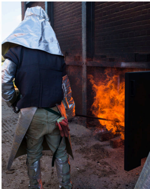
Figure 1: Drying and firing of bricks
