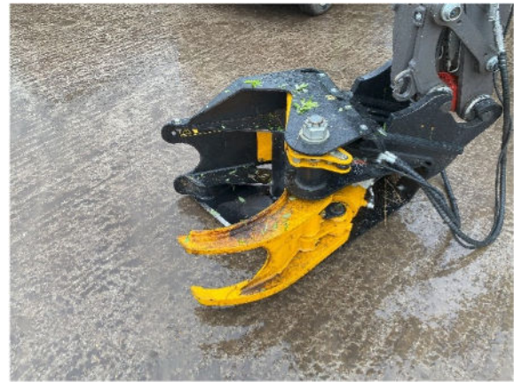
Figures 6 & 7: The willow is harvested with an excavator with a tree shear and grab attachment.
